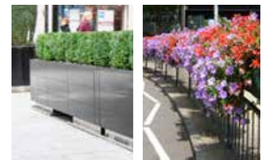
Examples of other simple SuDS retrofit measures - self irrigating planters
